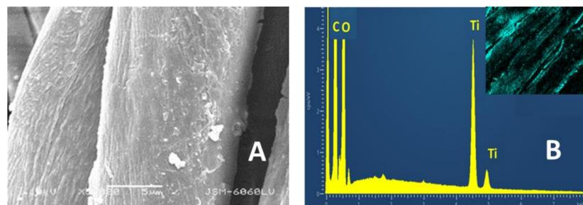
Figure 1. SEM image (A) and EDS spectrum (B) of CO( $\text{Ag}/\text{TiO}_2/\text{g-CN}$ ).
