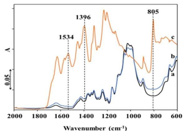
Figure 2. FTIR spectra of CO(UN) (a); CO( $\text{Ag}/\text{TiO}_2/\text{g-CN}$ ) (b); and  $\text{g-C}_3\text{N}_4$  powder (c).
