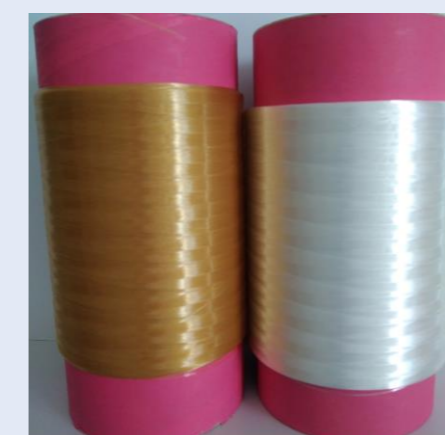
Figure 3. First modified PP with 10% myrrh and second pure PP multifilament yarns,
