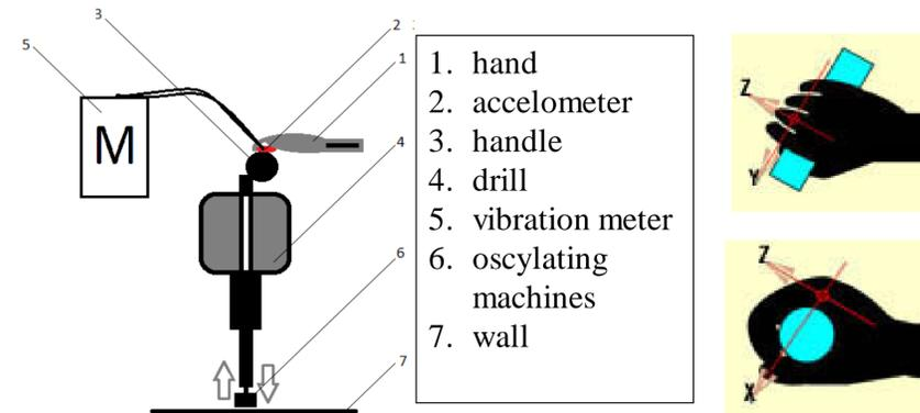
Fig.3. Scheme of the measuring stand; Coordinate systems used to measure hand vibration (ISO 5348)
