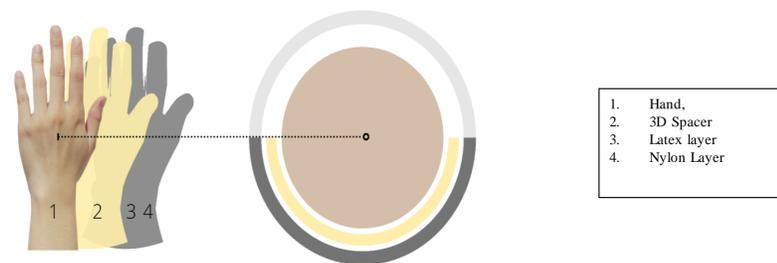
Fig. 2. The layout diagram in the prototype of an anti-vibration glove with a spacer knitted fabric insert
