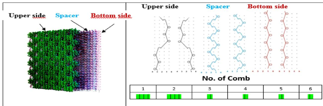
Fig. 1. Scheme of the structure of 3D knitted fabric; upper outer layer of spacer knit; fasteners; bottom layer of spacer knit. Gloves prototypes were made. The diagram of the arrangement of individual layers is shown in Fig. 2.
