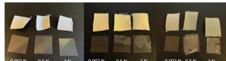
Figure 4. Adhesion test on fabric with circular cross-section 48 filaments. a) 90"; b) 120"; c) 300".
