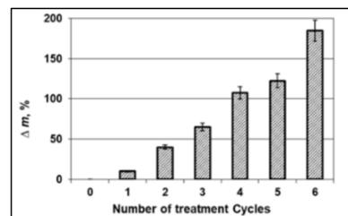
Figure 2. Influence of the number of treatment cycles on the fibres mass change [1].
