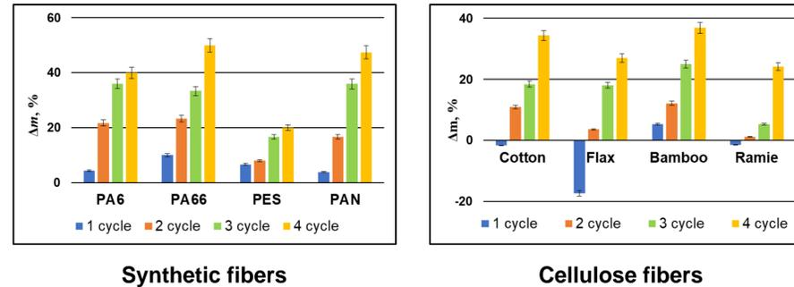
Figure 3. Variation in the mass of fibres of different nature during the process of modification with copper selenide
