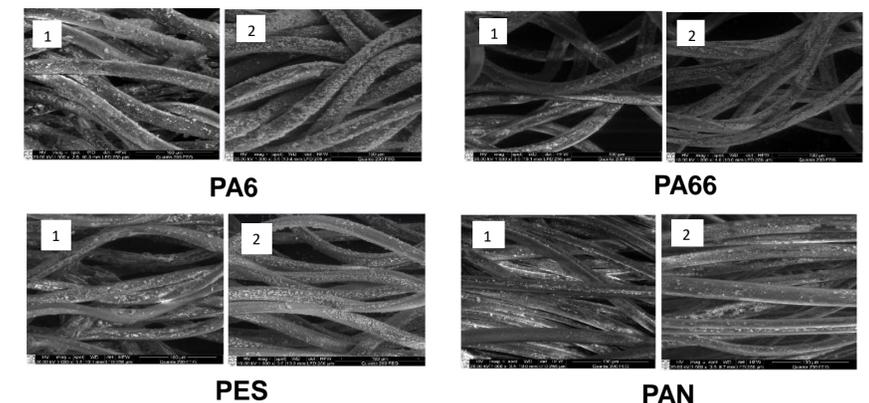
Figure 5. SEM images of copper selenide coated synthetic fibres after the second treatment cycle (mag. 1000×): 1 - after first treatment cycle, 2 - after second treatment cycle.
