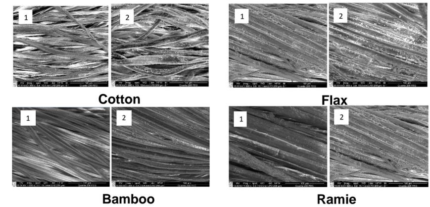
Figure 4. SEM images of copper selenide coated natural fibres after the first and fifth treatment cycle (mag. 1000×): 1 - after first treatment cycle, 2 - after second treatment cycle.
